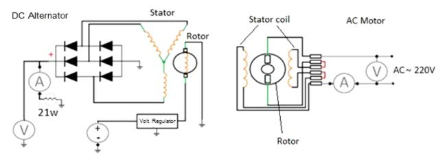
a) Scheme for measuring the parameters of the alternator when changing its revolutions and adding a load b) The scheme of the collector electric motor remains unchanged
