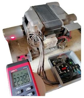
Fig. 10. Laser tachometer for non-contact measurement of revolutions
