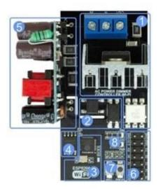
Fig. 7. Collector motor control module [https://robotdyn.com/ac-dimmer-controller-1channel-acesp8266.html]: 1) AC Dmmer 8A with RC filter; 2) AC Zero-cross detector; 3) WI-FI microcontroller ESP8266; 4) Flash memory 32MB (4MB); 5) AC-DC isolated power supply V<sub>DC</sub> = 3.3V (650mA); 6) Pinout 10 I/O header; 7) Buttons: Prog, Reset; 8) LED dimming indicate
