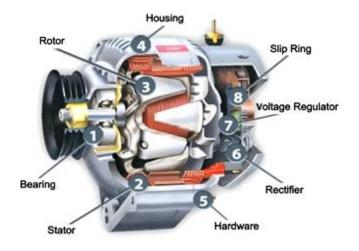
Fig. 1. Alternator components [https://engineeringlearn.com/alternator-definition-types-working-principleparts-uses-components-symptoms-of-bad-alternator]
