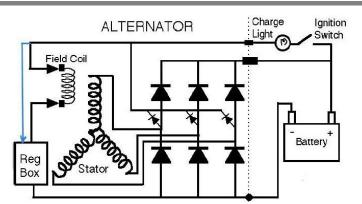
Fig. 2. Wiring diagram of the main components of the alternator [Borysiak, Moore, Sklar, Lamb, Dunn, p.15]
