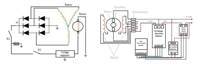
Fig. 6a. Alternator wiring diagram
