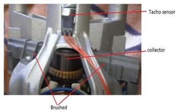
Fig. 4. The location of the collector, the location of the brush holders and the position of the sensor for measuring revolutions
